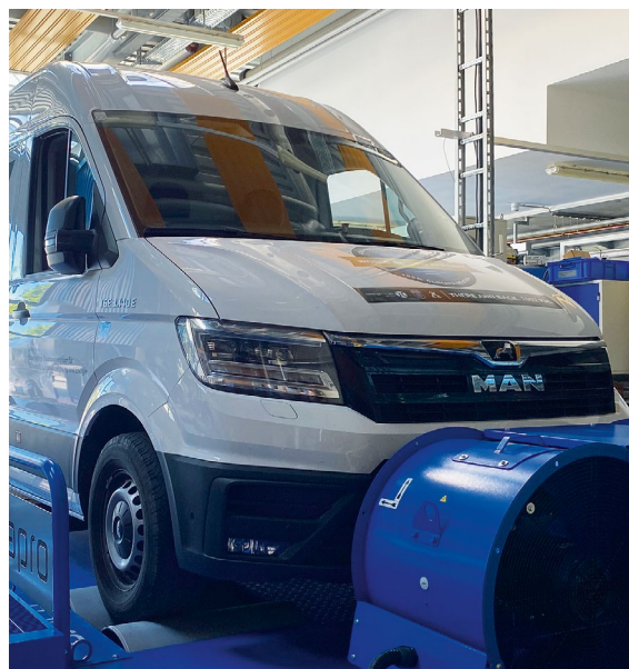
FIGURE 5 RMFC transporter prototype on the roller dynamometer (© Gumpert)
